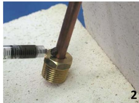
5. Some brazing/soldering joint designs may not have much of a "ledge" on which to deposit the paste. During heating of the part - and with gravity at work - the paste may run over the edge of the area on which it was placed. If this happens, use multiple deposits or apply a bead of paste to the part. You may also want to tilt the part slightly to direct the filler metal flow.
